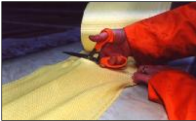
Cutting Kevlar ® fabric prior to wet lay up
