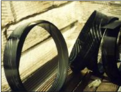
Pultruded plate is supplied in coils
